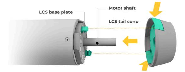
Install the LCS propeller using the same technique from Step 3. Depress the tabs, push the propeller onto the motor shaft, and rotate it until the LCS tabs click into place.
